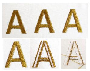
Too tight. Adjust the screw in quarter turns in an anticlockwise direction to loosen it.
