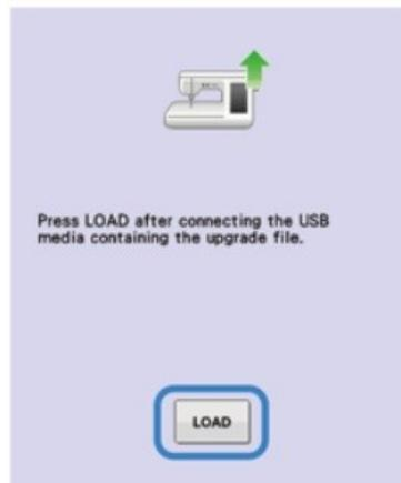
Wait until a screen appears saying the upgrade complete and then switch off the machine. Remove your USB flash drive and switch the machine back on. You can now check that the latest version has been installed by going back into the machine settings.
